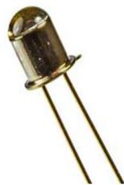
A typical phototransistor Note the lens at the top and the fact that it only has two leads because the base is often left open circuit and no external connection is provided.
